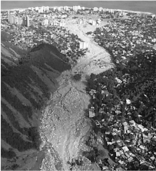
Figure 9. New stream channels and rocky debris on alluvial fan surface transported by flash floods and debris flows, Caraballeda, Venezuela.
